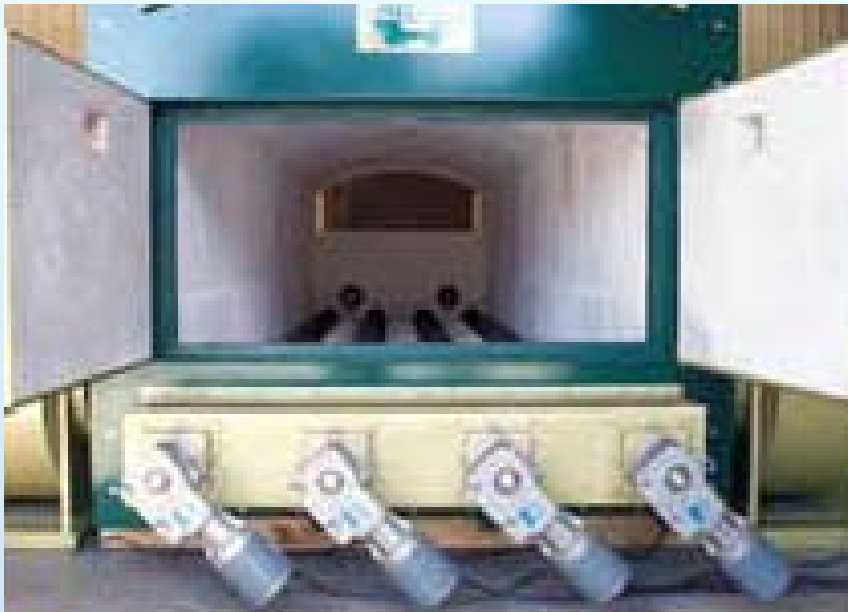
Inside of Combustion Unit
